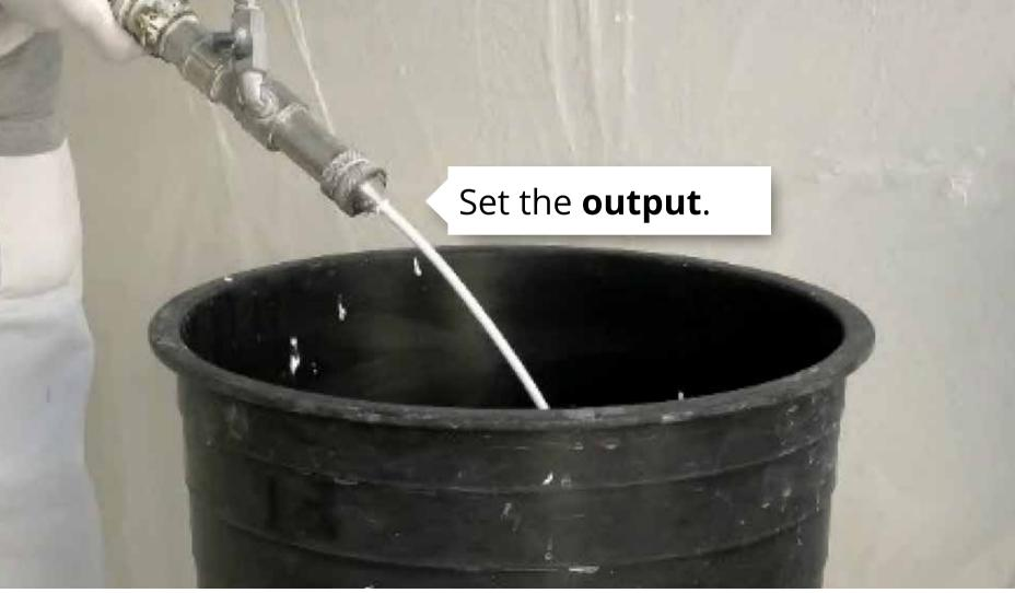
Then use a test surface to adjust the **spray pattern**, by adapting **air quantity** and output.
